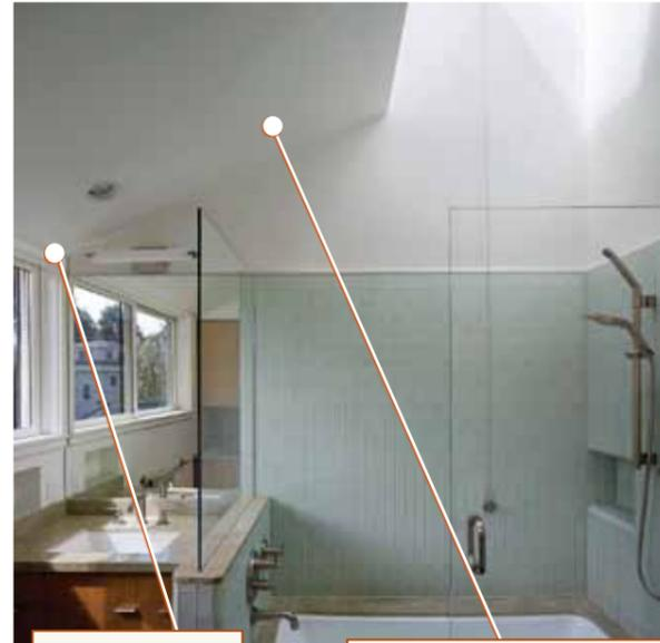
Bathrooms that have only one exterior wall and window can be a challenge to daylight properly. However, when the bathroom's ceiling is set just below the home's roofline—in a second-story bathroom, for example—I add a skylight to help balance the daylight.
